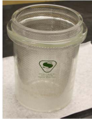
(b) Counter Electrode Inside the Cell
